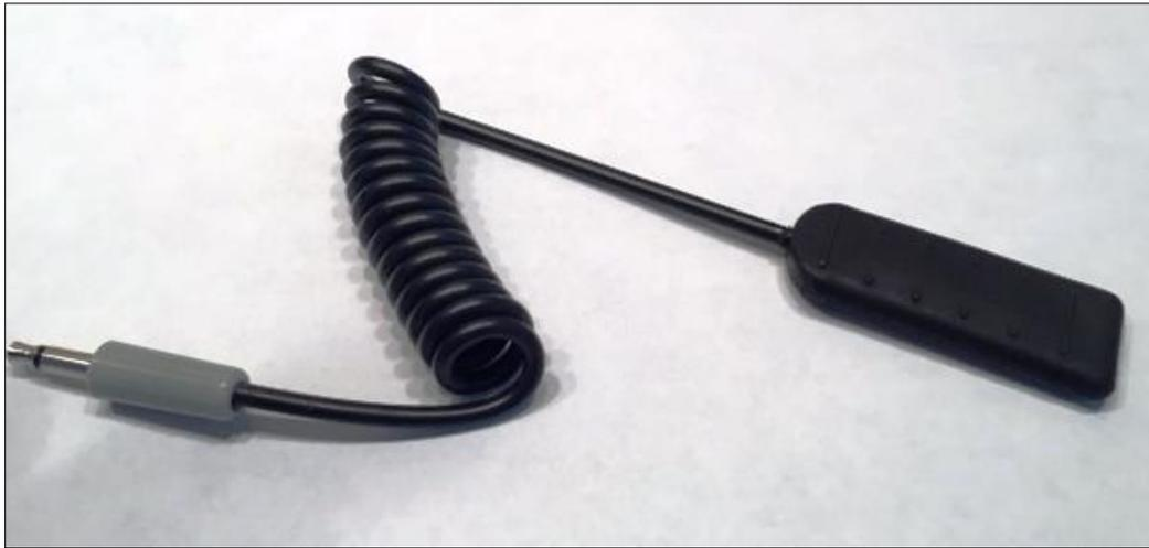
**Figure 5. Photograph of a SPST Switch Wire to a 3.5mm Plug for the PTT Function**
